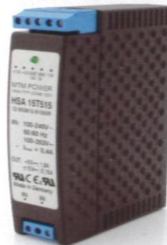
PCMed / PCMedmed encapsulated designs for medical applications are available in power ranges of from 15 watts – 100 watts. The primary voltage range of 90 -264 Vac / 100 -353 Vdc with single output selections for PCB and chassis mount applications where EN/UL 60 601-1/EN/UL 60 950-1 (2<sup>nd</sup> Edition) is necessary.
